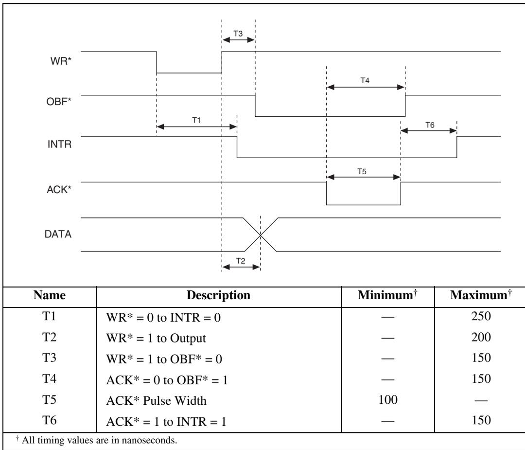
**Figure 4-3.** Timing Specifications for Mode 1 Output Transfer
