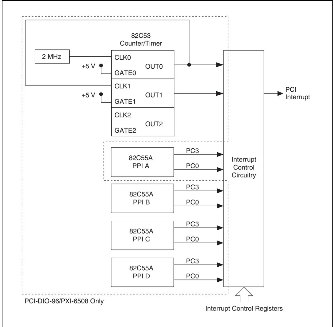
**Figure B-1.** Interrupt Control Circuitry Block Diagram
