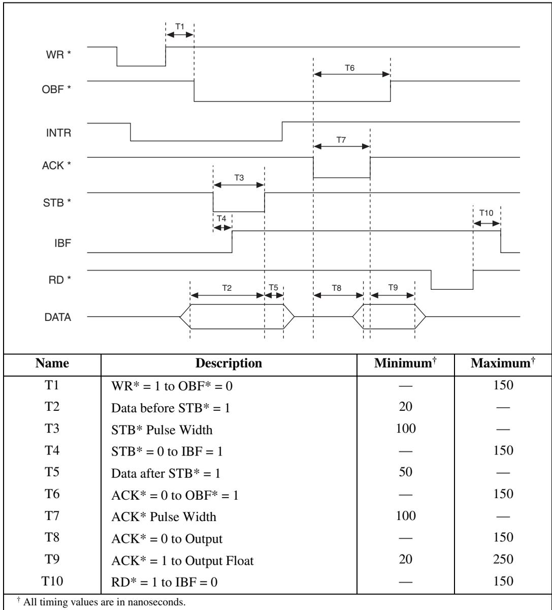
**Figure 4-4.** Timing Specifications for Mode 2 Bidirectional Transfer
